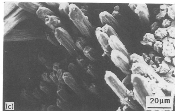
Figure 14 Lithium zinc silicate glass–ceramic/stainless steel filament reinforced composites, after [187]. (a) micrograph of sectioned composite containing 40 vol % continuous, aligned 22 \mu\text{m} diameter filaments; (b) fracture surface of similar 20 vol %, 22 \mu\text{m} composite; (c) fracture surface of similar 20 vol %, 8 \mu\text{m} composite.
