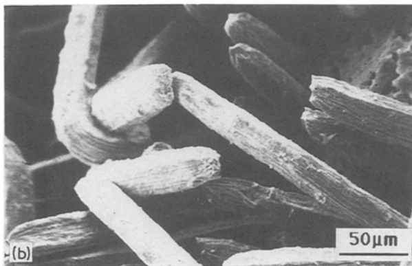
Figure 14 Lithium zinc silicate glass–ceramic/stainless steel filament reinforced composites, after [187]. (a) micrograph of sectioned composite containing 40 vol % continuous, aligned 22 \mu\text{m} diameter filaments; (b) fracture surface of similar 20 vol %, 22 \mu\text{m} composite; (c) fracture surface of similar 20 vol %, 8 \mu\text{m} composite.
